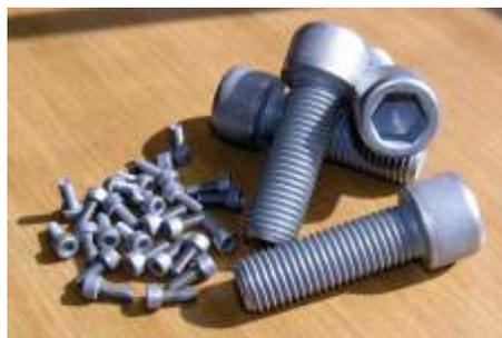
*Examples of mechanically plated metal fabrications (above) and Allen cap screws (below) processed at Team Plating Works*
